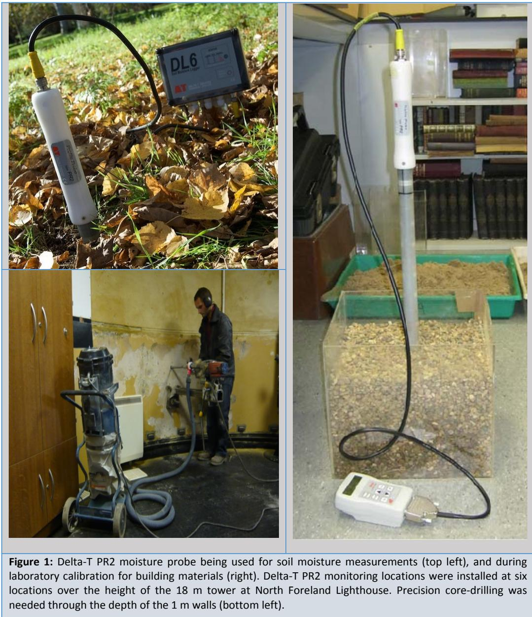
**Figure 1:** Delta-T PR2 moisture probe being used for soil moisture measurements (top left), and during laboratory calibration for building materials (right). Delta-T PR2 monitoring locations were installed at six locations over the height of the 18 m tower at North Foreland Lighthouse. Precision core-drilling was needed through the depth of the 1 m walls (bottom left).
